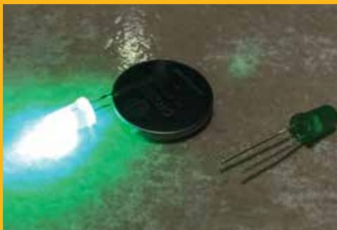
Grab two of your 5mm LED lights in the same color, and place them onto the coin battery. Here you will be completing a simple circuit. You will need to attach the positive side (+) of the light to the positive side of your battery, and the negative side (-) of your light to the negative side of your battery. (If the light doesn't light up, you will need to switch the sides) These are your bug's eyes!
