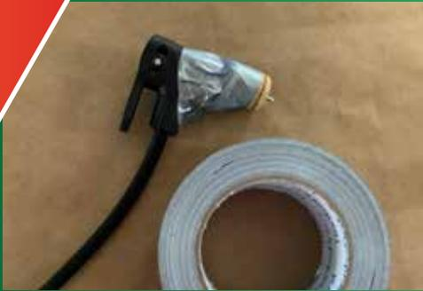
Secure your cork and inflating needle securely to the bike pump with tape.
