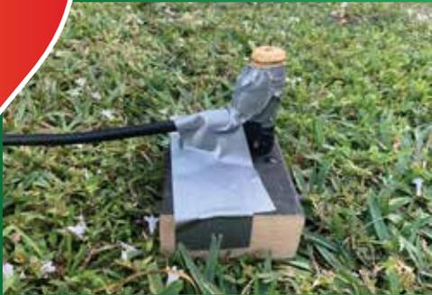
If not, use a small wooden block, rock, step, or anything outside to help keep the cork and inflating needle propped up. Secure these items to your pump, but still make sure the pump is not secured to the floor just yet.
