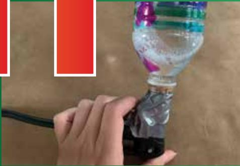
Place the cork attached to your pump inside your water bottle, making sure no water is leaking out.
