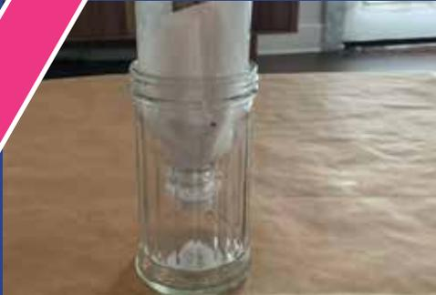
Place your cup or bottle inside a glass jar. This is your filtering system, so you should have some space in your jar for water to drain out of the bottom hole.
